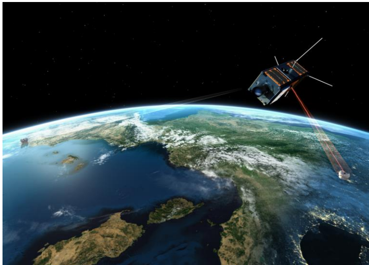
Laser Downlink Scenario from a miniaturized Transmitter Terminal on a CubeSat. Image Credits: DLR
