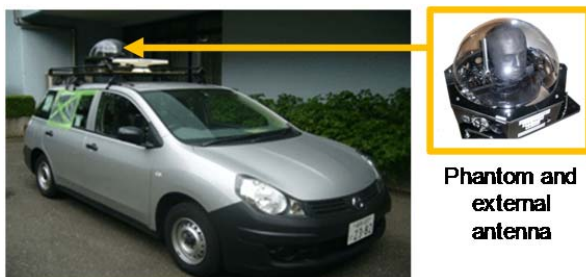
Figure 2. Test van for transmit power measurement.
