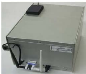
Figure 4. Prototype of multi-mode SDR VSAT IDU.
