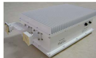
Figure 6. Prototype of integrated ODU/IDU.
