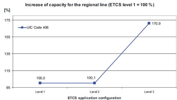
Fig. 7 Efficiency increase with moving blocks [4].
